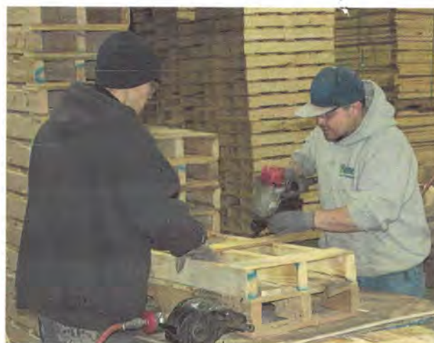
The pallet shop is well stocked for repair or custom work. Skilled workers build pallets to order from measurements taken by Chuck to provide stable shipping platforms for odd sized items.
