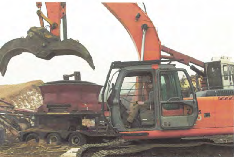
Two vital pieces of equipment for mulch making at Shelton's: a tracked Hitachi Zaxis 200 LC excavator, operated by Aaron Shelton, which loads the Toro tub grinder, shown in background.
